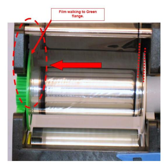
\*\*\*\*\* No gap between the film roll and the green flange. The film has started to spool up against the green flange (take-up spool).
