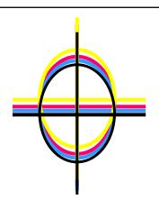
If **yellow appears below** magenta and magenta below cyan, as in the below picture, turn the bushing using a flat screwdriver to a setting toward **6** (o'clock)
